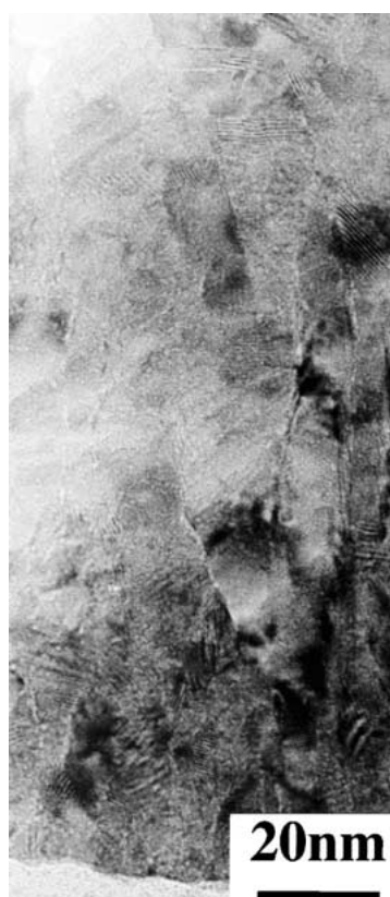
Figure 3 High resolution electron micrograph of a cross-sectional view of the iridium film deposited on graphite at the substrate temperature of 330 K.
